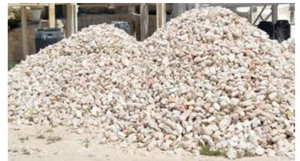
Rubble stones selected to go at the top of the kiln
